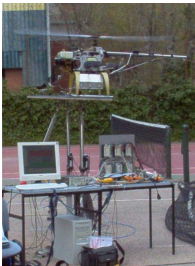
Fig. 4. Testbed: active helideck (AH) and ship platform (SP)
