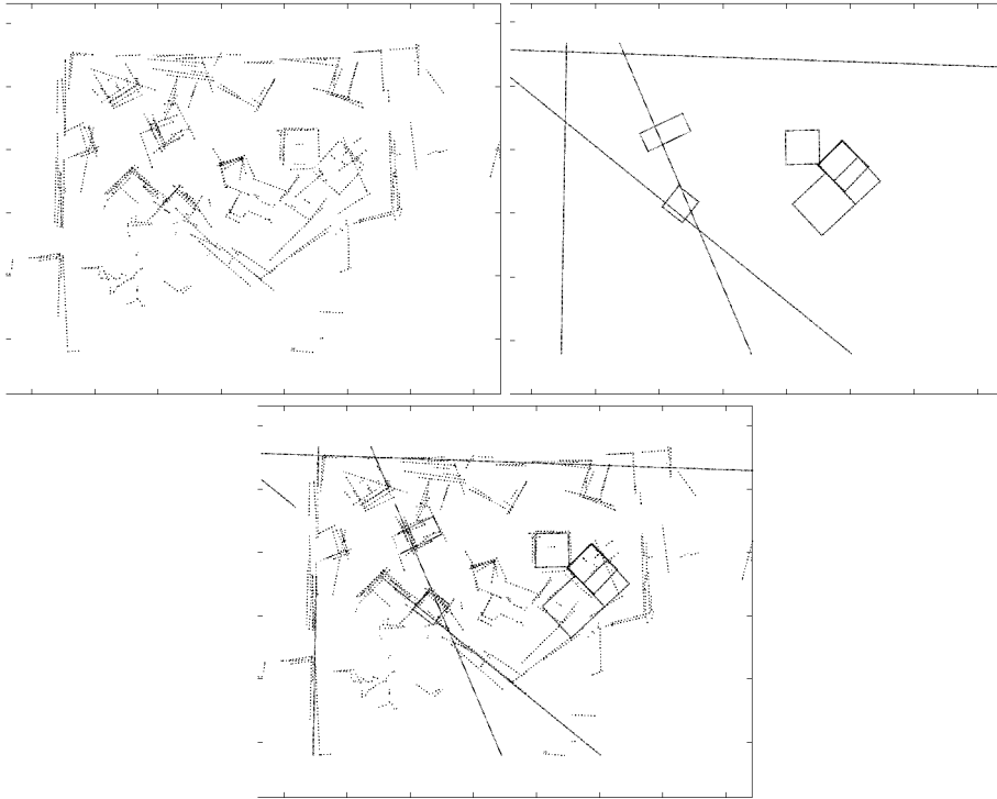
Fig. 8. Virtual Scans in an early stage of FFS. a) global map b) the Virtual Scan consisting of points representing detected lines and rectangles c) superimposition of real data and Virtual Scan. This is the data used in the next FFS iteration.
