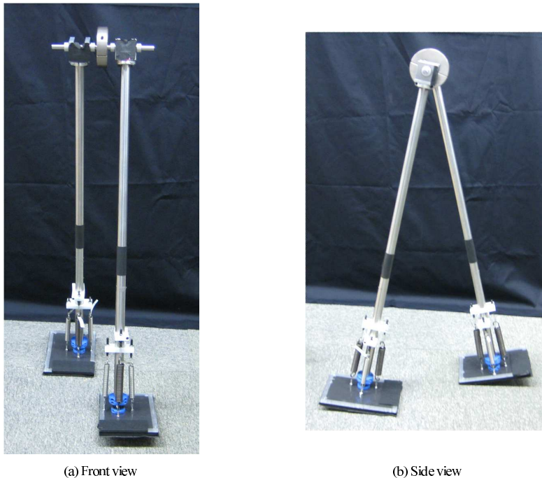
Fig. 11. A simple 3D straight-legged passive biped walker with flat feet and ankle springs.
